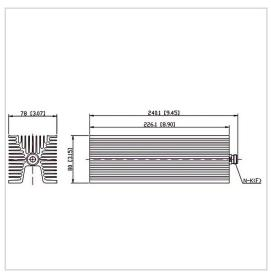
RF Solution offer a wide selection of Coaxial Fixed Termination (Dummy Load) for global customers. CT-200W-FA8022-NK-3G is Coaxial а Termination (Dummy Load) in Frequency Range of DC~3.0 GHz. It is made of high quality materials under a high standard, the Connector Type of this product is N-F (K), VSWR Max is 1.25 and Impedance is 50  $\Omega$ . The component has a good working performance and stability, it is ideal for handling a Power of 200 W.
