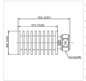
RF Solution offer a wide selection of Coaxial Fixed Termination (Dummy Load) for global customers. CT-20W-RA3657-4310J-3G is a Coaxial Fixed Termination (Dummy Load) in Frequency Range of DC~3.0 GHz. It is made of high quality materials under a high standard, the Connector Type of this product is 4.3-10-M (J), VSWR Max is 1.20 and Impedance is 50  $\Omega$ . The component has a good working performance and stability, it is ideal for handling a Power of 20 W.
