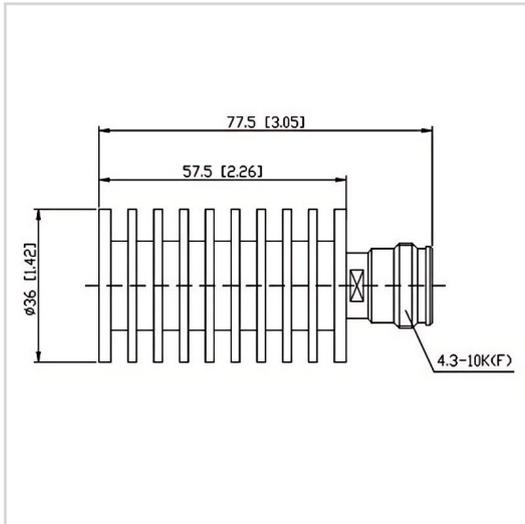
RF Solution offer a wide selection of Coaxial Fixed Termination (Dummy Load) for global customers. CT-20W-RA3657-4310K-3G is a Coaxial Fixed Termination (Dummy Load) in Frequency Range of DC~3.0 GHz. It is made of high quality materials under a high standard, the Connector Type of this product is 4.3-10-F (K), VSWR Max is 1.20 and Impedance is 50 Ω. The component has a good working performance and stability, it is ideal for handling a Power of 20 W.
