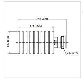
RF Solution offer a wide selection of Coaxial Fixed Termination (Dummy Load) for global customers. CT-20W-RA3657-4310K-4G is a Coaxial Fixed Termination (Dummy Load) in Frequency Range of DC~4.0 GHz. It is made of high quality materials under a high standard, the Connector Type of this product is 4.3-10-F (K), VSWR Max is 1.30 and Impedance is 50  $\Omega$ . The component has a good working performance and stability, it is ideal for handling a Power of 20 W.
