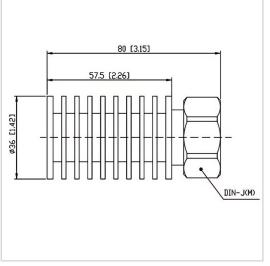
RF Solution offer a wide selection of Coaxial Fixed Termination (Dummy Load) for global customers. CT-20W-RA3657-DINJ-6G is а Coaxial Termination (Dummy Load) in Frequency Range of DC~6.0 GHz. It is made of high quality materials under a high standard, the Connector Type of this product is DIN-M (J), VSWR Max is 1.25 and Impedance is 50  $\Omega$ . The component has a good working performance and stability, it is ideal for handling a Power of 20 W.
