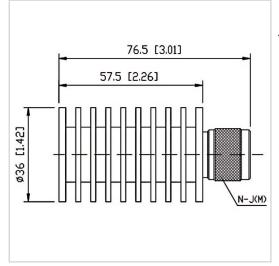
RF Solution offer a wide selection of Coaxial Fixed Termination (Dummy Load) for global customers. CT-20W-RA3657-NJ-4G is a Coaxial Fixed Termination (Dummy Load) in Frequency Range of DC~4.0 GHz. It is made of high quality materials under a high standard, the Connector Type of this product is N-M (J), VSWR Max is 1.20 and Impedance is 50  $\Omega$ . The component has a good working performance and stability, it is ideal for handling a Power of 20 W.
