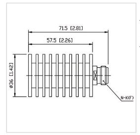
RF Solution offer a wide selection of Coaxial Fixed Termination (Dummy Load) for global customers. CT-20W-RA3657-NK-12.4G is a Coaxial Fixed Termination (Dummy Load) in Frequency Range of DC~12.4 GHz. It is made of high quality materials under a high standard, the Connector Type of this product is N-F (K), VSWR Max is 1.25 and Impedance is 50  $\Omega$ . The component has a good working performance and stability, it is ideal for handling a Power of 20 W.
