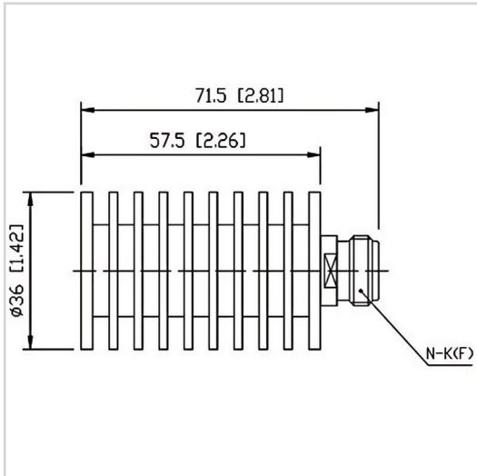
RF Solution offer a wide selection of Coaxial Fixed Termination (Dummy Load) for global customers. CT-20W-RA3657-NK-8G is a Coaxial Fixed Termination (Dummy Load) in Frequency Range of DC~8.0 GHz. It is made of high quality materials under a high standard, the Connector Type of this product is N-F (K), VSWR Max is 1.20 and Impedance is 50 Ω. The component has a good working performance and stability, it is ideal for handling a Power of 20 W.
