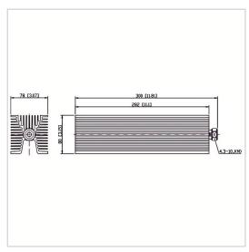
RF Solution offer a wide selection of Coaxial Fixed Termination (Dummy Load) for global customers. CT-300W-FA8028-4310J-3G is a Coaxial Fixed Termination (Dummy Load) in Frequency Range of DC~3.0 GHz. It is made of high quality materials under a high standard, the Connector Type of this product is 4.3-10-M (J), VSWR Max is 1.25 and Impedance is 50  $\Omega$ . The component has a good working performance and stability, it is ideal for handling a Power of 300 W.
