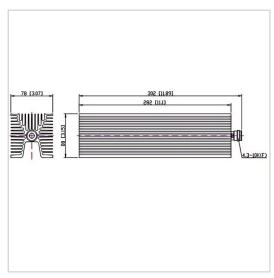
RF Solution offer a wide selection of Coaxial Fixed Termination (Dummy Load) for global customers. CT-300W-FA8028-4310K-4G is a Coaxial Fixed Termination (Dummy Load) in Frequency Range of DC~4.0 GHz. It is made of high quality materials under a high standard, the Connector Type of this product is 4.3-10-F (K), VSWR Max is 1.30 and Impedance is 50  $\Omega$ . The component has a good working performance and stability, it is ideal for handling a Power of 300 W.
