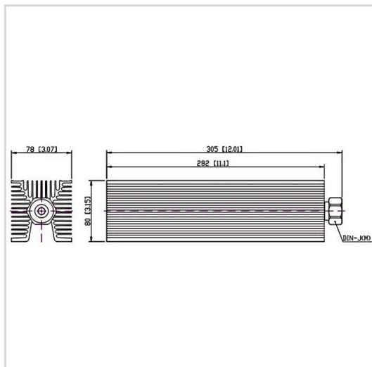
RF Solution offer a wide selection of Coaxial Fixed Termination (Dummy Load) for global customers. CT-300W-FA8028-DINJ-4G is a Coaxial Fixed Termination (Dummy Load) in Frequency Range of DC~4.0 GHz. It is made of high quality materials under a high standard, the Connector Type of this product is DIN-M (J), VSWR Max is 1.30 and Impedance is 50 Ω. The component has a good working performance and stability, it is ideal for handling a Power of 300 W.
