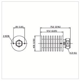
RF Solution offer a wide selection of Coaxial Fixed Termination (Dummy Load) for global customers. CT-30W-RA3857-4310J-4G is a Coaxial Fixed Termination (Dummy Load) in Frequency Range of DC~4.0 GHz. It is made of high quality materials under a high standard, the Connector Type of this product is 4.3-10-M (J), VSWR Max is 1.25 and Impedance is 50  $\Omega$ . The component has a good working performance and stability, it is ideal for handling a Power of 30 W.
