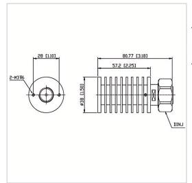
RF Solution offer a wide selection of Coaxial Fixed Termination (Dummy Load) for global customers. CT-30W-RA3857-DINJ-3G is a Coaxial Fixed Termination (Dummy Load) in Frequency Range of DC~3.0 GHz. It is made of high quality materials under a high standard, the Connector Type of this product is DIN-M (J), VSWR Max is 1.20 and Impedance is 50  $\Omega$ . The component has a good working performance and stability, it is ideal for handling a Power of 30 W.
