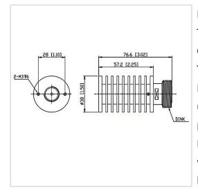
RF Solution offer a wide selection of Coaxial Fixed Termination (Dummy Load) for global customers. CT-30W-RA3857-DINK-4G is a Coaxial Fixed Termination (Dummy Load) in Frequency Range of DC~4.0 GHz. It is made of high quality materials under a high standard, the Connector Type of this product is DIN-F (K), VSWR Max is 1.25 and Impedance is 50  $\Omega$ . The component has a good working performance and stability, it is ideal for handling a Power of 30 W.
