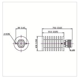
RF Solution offer a wide selection of Coaxial Fixed Termination (Dummy Load) for global customers. CT-30W-RA3857-NJ-12.4G is a Coaxial Fixed Termination (Dummy Load) in Frequency Range of DC~12.4 GHz. It is made of high quality materials under a high standard, the Connector Type of this product is N-M (J), VSWR Max is 1.30 and Impedance is 50  $\Omega$ . The component has a good working performance and stability, it is ideal for handling a Power of 30 W.
