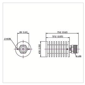
RF Solution offer a wide selection of Coaxial Fixed Termination (Dummy Load) for global customers. CT-30W-RA3857-NJ-18G is a Coaxial Fixed Termination (Dummy Load) in Frequency Range of DC~18.0 GHz. It is made of high quality materials under a high standard, the Connector Type of this product is N-M (J), VSWR Max is 1.35 and Impedance is 50  $\Omega$ . The component has a good working performance and stability, it is ideal for handling a Power of 30 W.
