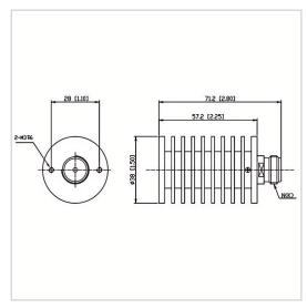
RF Solution offer a wide selection of Coaxial Fixed Termination (Dummy Load) for global customers. CT-30W-RA3857-NK-4G is Coaxial Fixed а Termination (Dummy Load) in Frequency Range of DC~4.0 GHz. It is made of high quality materials under a high standard, the Connector Type of this product is N-F (K), VSWR Max is 1.20 and Impedance is 50  $\Omega$ . The component has a good working performance and stability, it is ideal for handling a Power of 30 W.
