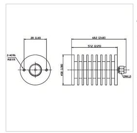
RF Solution offer a wide selection of Coaxial Fixed Termination (Dummy Load) for global customers. CT-30W-RA3857-SJ-8G is a Coaxial Fixed Termination (Dummy Load) in Frequency Range of DC~8.0 GHz. It is made of high quality materials under a high standard, the Connector Type of this product is SMA-M (J), VSWR Max is 1.30 and Impedance is 50  $\Omega$ . The component has a good working performance and stability, it is ideal for handling a Power of 30 W.
