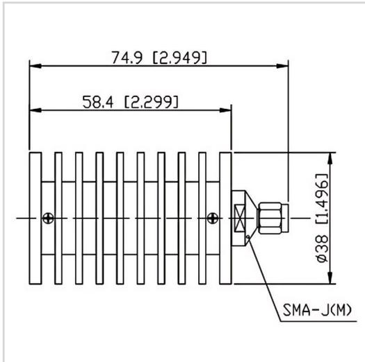
RF Solution offer a wide selection of Coaxial Fixed Termination (Dummy Load) for global customers. CT-30W-RA3858-SJ-10G is a Coaxial Fixed Termination (Dummy Load) in Frequency Range of DC~10.0 GHz. It is made of high quality materials under a high standard, the Connector Type of this product is SMA-M (J), VSWR Max is 1.30 and Impedance is 50 Ω. The component has a good working performance and stability, it is ideal for handling a Power of 30 W.
