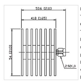
RF Solution offer a wide selection of Coaxial Fixed Termination (Dummy Load) for global customers. CT-30W-RA5442-2.92J-40G is a Coaxial Fixed Termination (Dummy Load) in Frequency Range of DC~40.0 GHz. It is made of high quality materials under a high standard, the Connector Type of this product is 2.92-M (J), VSWR Max is 1.30 and Impedance is 50  $\Omega$ . The component has a good working performance and stability, it is ideal for handling a Power of 30 W.
