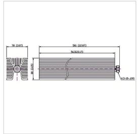
RF Solution offer a wide selection of Coaxial Fixed Termination (Dummy Load) for global customers. CT-500W-FA8056-4310J-3G is a Coaxial Fixed Termination (Dummy Load) in Frequency Range of DC~3.0 GHz. It is made of high quality materials under a high standard, the Connector Type of this product is 4.3-10-M (J), VSWR Max is 1.30 and Impedance is 50  $\Omega$ . The component has a good working performance and stability, it is ideal for handling a Power of 500 W.
