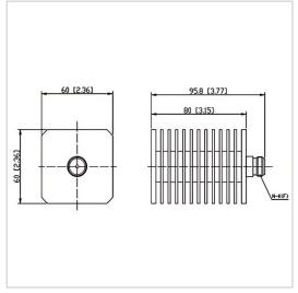
RF Solution offer a wide selection of Coaxial Low PIM Termination for global customers. CT-50W-FH6080-IP65-NK-3G is a Coaxial Low PIM Termination in Frequency Range of DC $\sim$ 3.0 GHz. It is made of high quality materials under a high standard, the Connector Type of this product is N-F (K), VSWR Max is 1.20 and Impedance is 50  $\Omega$ . The component has a good working performance and stability, it is ideal for handling a Power of 50 W.
