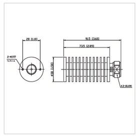
RF Solution offer a wide selection of Coaxial Fixed Termination (Dummy Load) for global customers. CT-50W-RA3873-4310J-4G is a Coaxial Fixed Termination (Dummy Load) in Frequency Range of DC~4.0 GHz. It is made of high quality materials under a high standard, the Connector Type of this product is 4.3-10-M (J), VSWR Max is 1.25 and Impedance is 50  $\Omega$ . The component has a good working performance and stability, it is ideal for handling a Power of 50 W.
