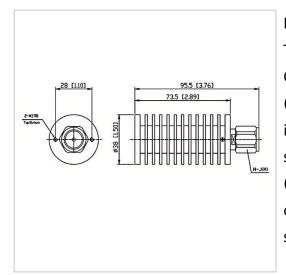
RF Solution offer a wide selection of Coaxial Fixed Termination (Dummy Load) for global customers. CT-50W-RA3873-NJ-8G is a Coaxial Fixed Termination (Dummy Load) in Frequency Range of DC~8.0 GHz. It is made of high quality materials under a high standard, the Connector Type of this product is N-M (J), VSWR Max is 1.30 and Impedance is 50  $\Omega$ . The component has a good working performance and stability, it is ideal for handling a Power of 50 W.
