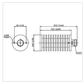
RF Solution offer a wide selection of Coaxial Fixed Termination (Dummy Load) for global customers. CT-50W-RA3873-NK-6G is a Coaxial Fixed Termination (Dummy Load) in Frequency Range of DC $\sim$ 6.0 GHz. It is made of high quality materials under a high standard, the Connector Type of this product is N-F (K), VSWR Max is 1.25 and Impedance is 50  $\Omega$ . The component has a good working performance and stability, it is ideal for handling a Power of 50 W.
