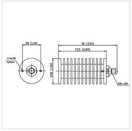
RF Solution offer a wide selection of Coaxial Fixed Termination (Dummy Load) for global customers. CT-50W-RA3873-SJ-3G is a Coaxial Fixed Termination (Dummy Load) in Frequency Range of DC~3.0 GHz. It is made of high quality materials under a high standard, the Connector Type of this product is SMA-M (J), VSWR Max is 1.20 and Impedance is 50  $\Omega$ . The component has a good working performance and stability, it is ideal for handling a Power of 50 W.
