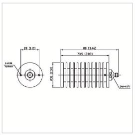
RF Solution offer a wide selection of Coaxial Fixed Termination (Dummy Load) for global customers. CT-50W-RA3873-SK-3G is a Coaxial Fixed Termination (Dummy Load) in Frequency Range of DC $\sim$ 3.0 GHz. It is made of high quality materials under a high standard, the Connector Type of this product is SMA-F (K), VSWR Max is 1.20 and Impedance is 50  $\Omega$ . The component has a good working performance and stability, it is ideal for handling a Power of 50 W.
