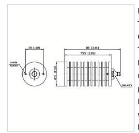
RF Solution offer a wide selection of Coaxial Fixed Termination (Dummy Load) for global customers. CT-50W-RA3873-SK-8G is a Coaxial Fixed Termination (Dummy Load) in Frequency Range of DC~8.0 GHz. It is made of high quality materials under a high standard, the Connector Type of this product is SMA-F (K), VSWR Max is 1.30 and Impedance is 50  $\Omega$ . The component has a good working performance and stability, it is ideal for handling a Power of 50 W.
