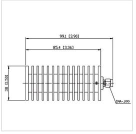
RF Solution offer a wide selection of Coaxial Fixed Termination (Dummy Load) for global customers. CT-50W-RA3885-SJ-10G is a Coaxial Fixed Termination (Dummy Load) in Frequency Range of DC~10.0 GHz. It is made of high quality materials under a high standard, the Connector Type of this product is SMA-M (J), VSWR Max is 1.30 and Impedance is 50  $\Omega$ . The component has a good working performance and stability, it is ideal for handling a Power of 50 W.
