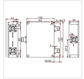
RF Solution offer a wide selection of RF Duplexer for global customers. DUP-1150M1530-150A100S is a RF Duplexer in Frequency Range of 1150~1630 MHz. It is made of high quality materials under a high standard, the Insertion Loss Max of this product is 0.4 dB, Ripple Max is 0.3 dB and Return Loss Min is 18 dB. The component has a good working performance and stability, it is ideal for handling a Power Rating of 100 W.
