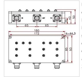
RF Solution offer a wide selection of RF Duplexer for global customers. DUP-1215M1550-46A60NA is a RF Duplexer in Frequency Range of 1215~1610 MHz. It is made of high quality materials under a high standard, the Insertion Loss Max of this product is 0.3 dB, Ripple Max is 0.2 dB and Return Loss Min is 18 dB. The component has a good working performance and stability, it is ideal for handling a Power Rating of 300 W.
