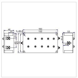
RF Solution offer a wide selection of RF Duplexer for global customers. DUP-450M758-50A107S is a RF Duplexer in Frequency Range of 450~865 MHz. It is made of high quality materials under a high standard, the Insertion Loss Max of this product is 0.5 dB, Ripple Max is 0.3 dB and Return Loss Min is 18 dB. The component has a good working performance and stability, it is ideal for handling a Power Rating of 5 W.
