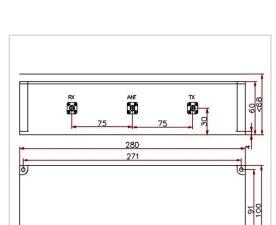
RF Solution offer a wide selection of RF Duplexer for global customers. DUP-457M467-02S is a RF Duplexer in Frequency Range of 457~469 MHz. It is made of high quality materials under a high standard, the Insertion Loss Max of this product is 2.0 dB, Ripple Max is 0.6 dB and Return Loss Min is 18 dB. The component has a good working performance and stability, it is ideal for handling a Power Rating of 50 W.
