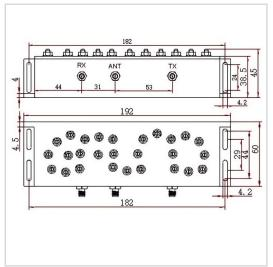
RF Solution offer a wide selection of RF Duplexer for global customers. DUP-824M869-25S is a RF Duplexer in Frequency Range of 824~894 MHz. It is made of high quality materials under a high standard, the Insertion Loss Max of this product is 1.5 dB, Ripple Max is 1.0 dB and Return Loss Min is 18 dB. The component has a good working performance and stability, it is ideal for handling a Power Rating of 50 W.
