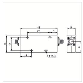
RF Solution offer a wide selection of High Pass Filter for global customers. HPF-1.5G14A-S is a High Pass Filter in Frequency Range of 1.5~14.0 GHz. It is made of high quality materials under a high standard, the Insertion Loss Max of this product is 1.5dB@1500-1600MHz / 1.0dB@1600-14000MHz, Rejection Min is 50dB@DC-1170MHz and VSWR Max is 1.50. The component has a good working performance and stability, it is ideal for handling a Rated Power of 15 W.
