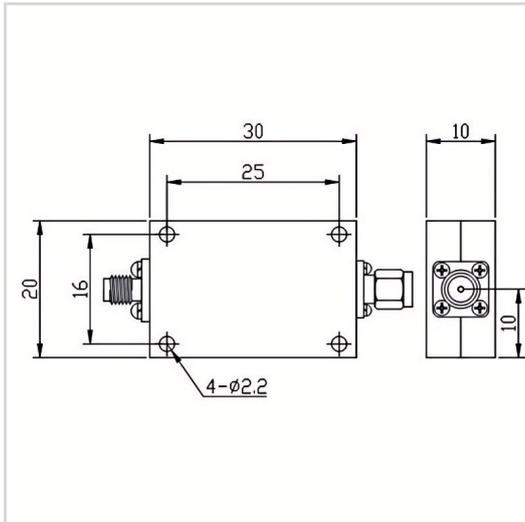
RF Solution offer a wide selection of High Pass Filter for global customers. HPF-11.7G15A-S is a High Pass Filter in Frequency Range of 11.7~15.0 GHz. It is made of high quality materials under a high standard, the Insertion Loss Max of this product is 1.0 dB, Rejection Min is 15dB@DC-9.8GHz and VSWR Max is 1.30. The component has a good working performance and stability, it is ideal for handling a Rated Power of 10 W.
