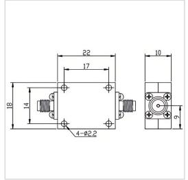
RF Solution offer a wide selection of High Pass Filter for global customers. HPF-11G24A-S is a High Pass Filter in Frequency Range of 11.0~24.0 GHz. It is made of high quality materials under a high standard, the Insertion Loss Max of this product is 2.5 dB, Rejection Min is 60dB@DC-6000MHz / 40dB@6000-9000MHz and VSWR Max is 1.80. The component has a good working performance and stability, it is ideal for handling a Rated Power of 10 W.
