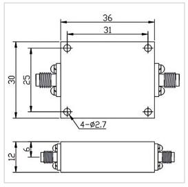
RF Solution offer a wide selection of High Pass Filter for global customers. HPF-2.4835G18A-S is a High Pass Filter in Frequency Range of 2.4835~18.0 GHz. It is made of high quality materials under a high standard, the Insertion Loss Max of this product is 2.0 dB, Rejection Min is 60dB@DC-1664MHz and VSWR Max is 2.00. The component has a good working performance and stability, it is ideal for handling a Rated Power of 20 W.
