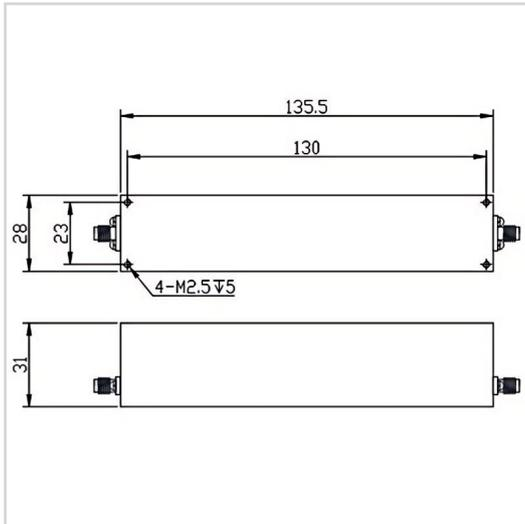
RF Solution offer a wide selection of High Pass Filter for global customers. HPF-2.65G7.5A-S is a High Pass Filter in Frequency Range of 2650~7500 MHz. It is made of high quality materials under a high standard, the Insertion Loss Max of this product is 1.8 dB, Rejection Min is 70dB@DC-2450MHz and VSWR Max is 2.00. The component has a good working performance and stability, it is ideal for handling a Rated Power of 20 W.
