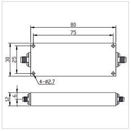
RF Solution offer a wide selection of High Pass Filter for global customers. HPF-2.7835G18A-S is a High Pass Filter in Frequency Range of 2.7835~18.0 GHz. It is made of high quality materials under a high standard, the Insertion Loss Max of this product is 1.8 dB, Rejection Min is 70dB@DC-2.4835GHz and VSWR Max is 2.00. The component has a good working performance and stability, it is ideal for handling a Rated Power of 20 W.
