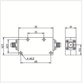
RF Solution offer a wide selection of High Pass Filter for global customers. HPF-3.1G18A-S is a High Pass Filter in Frequency Range of 3.1~18.0 GHz. It is made of high quality materials under a high standard, the Insertion Loss Max of this product is 1.50 dB, Rejection Min is 50dB@DC-2.48GHz and VSWR Max is 1.50. The component has a good working performance and stability, it is ideal for handling a Rated Power of 10 W.
