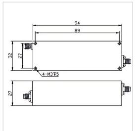
RF Solution offer a wide selection of High Pass Filter for global customers. HPF-4.492G18A-S is a High Pass Filter in Frequency Range of 4.492~18.0 GHz. It is made of high quality materials under a high standard, the Insertion Loss Max of this product is 2.0 dB, Rejection Min is 40dB@DC-4.2GHz and VSWR Max is 2.00. The component has a good working performance and stability, it is ideal for handling a Rated Power of 20 W.
