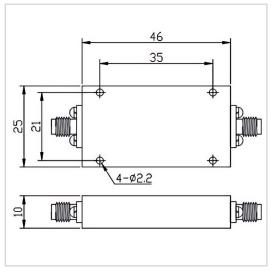
RF Solution offer a wide selection of High Pass Filter for global customers. HPF-4G18A-S is a High Pass Filter in Frequency Range of 4.0~18.0 GHz. It is made of high quality materials under a high standard, the Insertion Loss Max of this product is 1.50 dB, Rejection Min is 2.0dB@4000-4400MHz / 1.0dB@4400-18000MHz and VSWR Max is 1.80. The component has a good working performance and stability, it is ideal for handling a Rated Power of 20 W.
