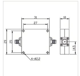
RF Solution offer a wide selection of High Pass Filter for global customers. HPF-6.5G18A-S is a High Pass Filter in Frequency Range of 6.5~18.0 GHz. It is made of high quality materials under a high standard, the Insertion Loss Max of this product is 2.0 dB, Rejection Min is 40@5850MHz / 62@DC-5590MHZ and VSWR Max is 1.80. The component has a good working performance and stability, it is ideal for handling a Rated Power of 20 W.
