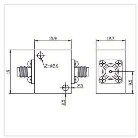
RF Solution offer a wide selection of High Pass Filter for global customers. HPF-6G18A-S is a High Pass Filter in Frequency Range of 6.0~18.0 GHz. It is made of high quality materials under a high standard, the Insertion Loss Max of this product is 1.0 Rejection Min 50dB@DC-613MHz is 25dB@2500MHz and VSWR Max is 2.00. The component has a good working performance and stability, it is ideal for handling a Rated Power of 10 W.
