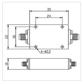
RF Solution offer a wide selection of High Pass Filter for global customers. HPF-6G24A-S is a High Pass Filter in Frequency Range of 6.0~24.0 GHz. It is made of high quality materials under a high standard, the Insertion Loss Max of this product is 2.0 dB, Rejection Min is 60dB@DC-5400MHz and VSWR Max is 1.80. The component has a good working performance and stability, it is ideal for handling a Rated Power of 15 W.
