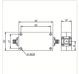
RF Solution offer a wide selection of High Pass Filter for global customers. HPF-7G18A-S is a High Pass Filter in Frequency Range of 7.0~18.0 GHz. It is made of high quality materials under a high standard, the Insertion Loss Max of this product is 2.0 dB, Rejection Min is 40dB@DC-6.5GHZ and VSWR Max is 2.00. The component has a good working performance and stability, it is ideal for handling a Rated Power of 10 W.
