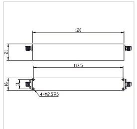
RF Solution offer a wide selection of High Pass Filter for global customers. HPF-8.4G17A-S is a High Pass Filter in Frequency Range of 8.4~17.0 GHz. It is made of high quality materials under a high standard, the Insertion Loss Max of this product is 2.0 dB, Rejection Min is 5.0dB@8400-8450MHz / 3.0dB@8450-17000MHz and VSWR Max is 1.50. The component has a good working performance and stability, it is ideal for handling a Rated Power of 35 W.
