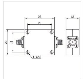
RF Solution offer a wide selection of High Pass Filter for global customers. HPF-8G18A-S is a High Pass Filter in Frequency Range of 8.0~18.0 GHz. It is made of high quality materials under a high standard, the Insertion Loss Max of this product is 2.0 dB, Rejection Min is 50dB@DC-6800MHZ and VSWR Max is 2.00. The component has a good working performance and stability, it is ideal for handling a Rated Power of 5 W.
