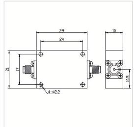
RF Solution offer a wide selection of High Pass Filter for global customers. HPF-8G25A-S is a High Pass Filter in Frequency Range of 8.0~25.0 GHz. It is made of high quality materials under a high standard, the Insertion Loss Max of this product is 2.0 dB, Rejection Min is 2.0dB@8000-8500MHz / 1.0dB@8500-25000MHz and VSWR Max is Input 1.50 Output 1.50. The component has a good working performance and stability, it is ideal for handling a Rated Power of 15 W.
